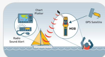
The MOB1 is intended to be installed within the lifejacket and will activate automatically on inflation, sending the first alert within 15 seconds. The MOB1 is waterproof to 10 metres.
